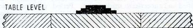
FIG. 12. Octagonally shaped device, which, when fitted above table level, cuts up the leaf
