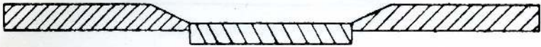
FIG. 1. Section of early type of roller table with concave door and no battens.
