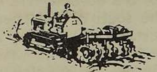
BUSH AND BOG HARROWS work among stumps, over rough terrain.
