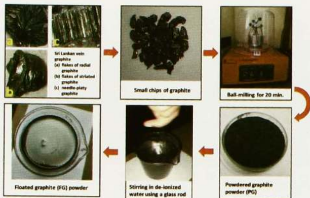
Figure 1: The process flow diagram of obtaining floated graphite from Sri Lankan vein graphite.
