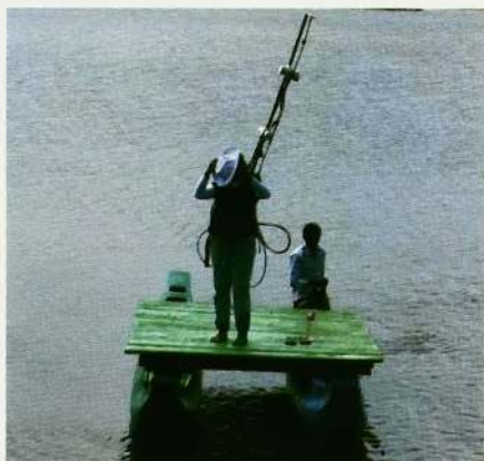
Fig 1: Conducting magnetic survey in Nelum Wewa using a portable magnetometer.
