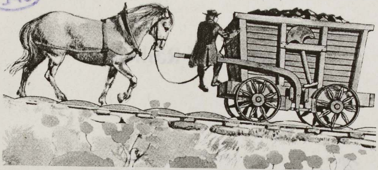
Loded Coal Wagon Coasting downhill. The horse will haul it back
