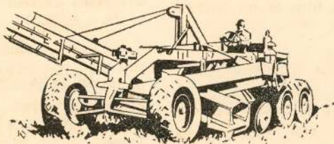
DOMOR —elevating grader attachment for Caterpillar Motor Graders, rotary snow plows, road wideners.
