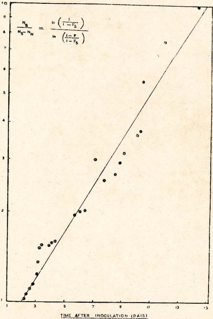
Fig. 6 CHANGE OF THE RECIPROCAL OF THE FRACTIONAL DEVIATION FROM SATURATION \frac{N_s}{N_s - N_t} WITH TIME (t)
