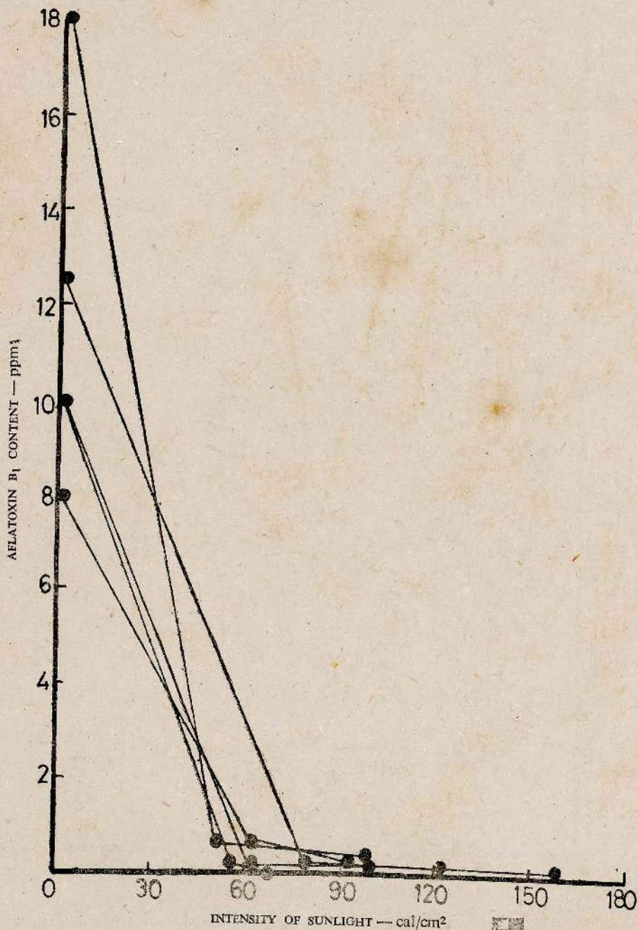
Figure II. Effect of exposure to sunlight, on the aflatoxin B 1 content of experimentally contaminated coconut oil containing high levels of toxin. ●—● = replicate samples.
