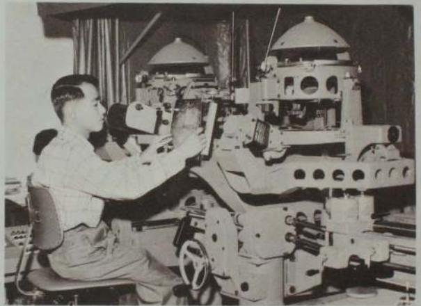
North Borneo trainee, schooled in Australia, operates photo plotting machine which produces maps from aerial photographs.
