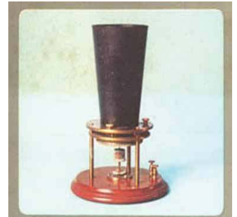
1876 LIQUID TELEPHONE "Mr. Watson, come here; I want you!" These historic words, the first articulate sentence ever spoken over an electric telephone, were uttered by Alexander Graham Bell when he spilled on his clothes some sulphuric acid which was part of the transmission apparatus. It was the night of March 10, 1876. The receiver was a tuned reed.
