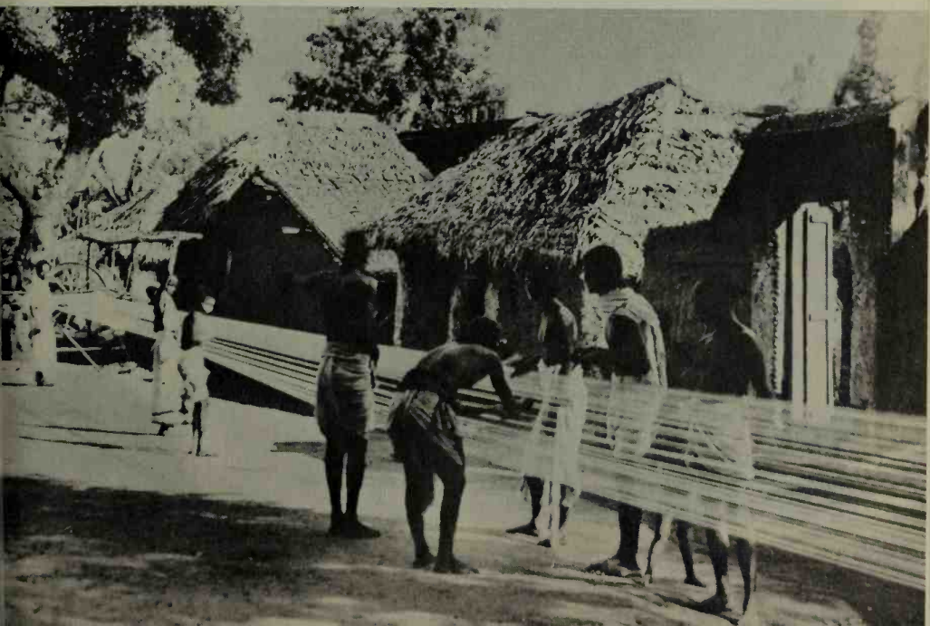
35. Laying a warp in Madura.
