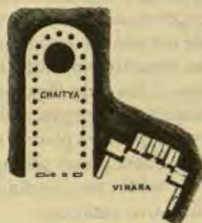
Plan of chaitya -cave and vihara , Bhaja. After Fergusson. Scale 50 feet to 1 inch.
