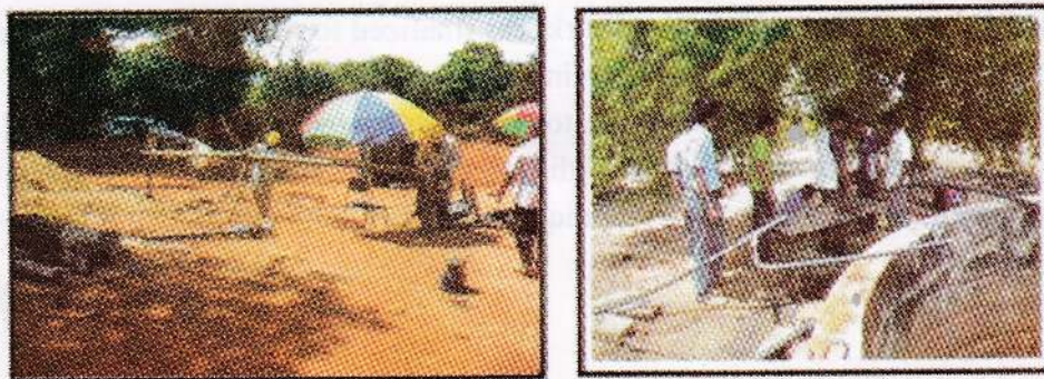
Figure: Test pumping done at Iyakachchi area. Test pumping carried out at different aquifer types in the area and the analyses results of those tests were used to estimate the aquifer parameters & characteristics.
