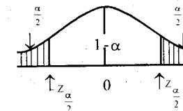
$$P\left(-z_{\alpha/2} < \frac{\bar{x} - \mu}{\sigma/\sqrt{n}} < z_{\alpha/2}\right) = 1 - \alpha$$
