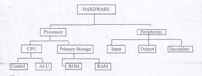
As mentioned above the data processing unit (CPU and primary storage) and all the other perpheral equipments connected to all refereed to as HARDWARE OF THE SYSTEM.
